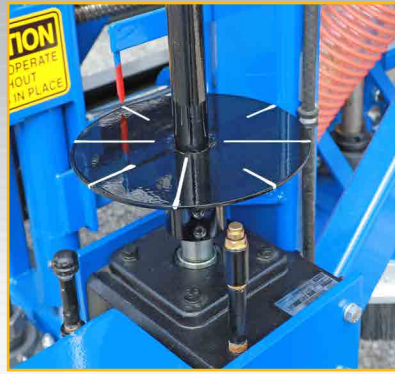
Indicator Wheel used by operator when micro-adjusting the cutterhead vertically when sanding.
