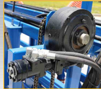
Viewing Hydraulic Motor and Gear Reducer, used to power Slab Surfacers along track.
