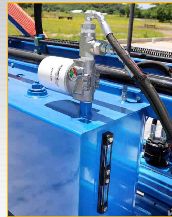
Viewing 90 Gallon Hydraulic Oil Reservoir with Return Filter and Oil Level Temperature Gauge
