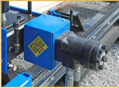
Hydraulic motor powers a 20-1 Gear Reducer for powerlift of Cutterhead.
