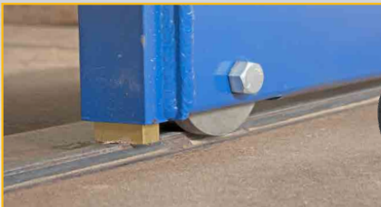
Hardened Casters and Bronze Track Scrapers on 3/4" x 3/4" Rail
